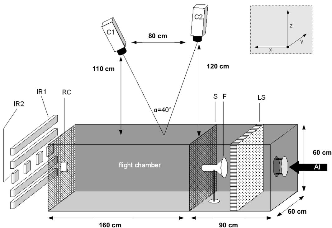
**Figure 1.** Wind tunnel set-up. Air inlet (AI), lamination screen (LS), glass funnel containing heat element (F), mesh screen (S), release cup (RC), cameras (C1,2), IR lights type 1 (IR1), IR lights type 2 (IR2). Mosquitoes were in view of both cameras up to 60 cm downwind from the mesh screen (S).
