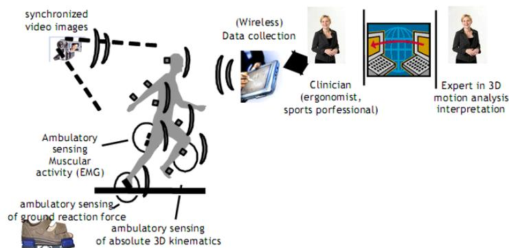
**Figure 1.** FreeMotion concept for ambulatory 3D analysis of human movement combining body worn inertial sensors for kinematics, force and EMG, wireless video streams real-time wireless recording and data representation, and modern internet support.
