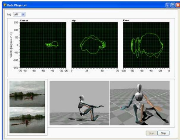
**Figure 3.** Example in sports coaching (here varsity rowing), where a sports coach is assisted in real-time monitoring 3D posture, movement and timing of a rower on the water. The coach can view the rower's motion from all sides and study specific timing and kinematics parameters. 2 wireless video streams provide context awareness.
