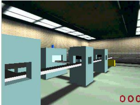
The user navigates through a virtual factory with a prototype of a new production line. Meanwhile, the Virtual Observer records all relevant events.
