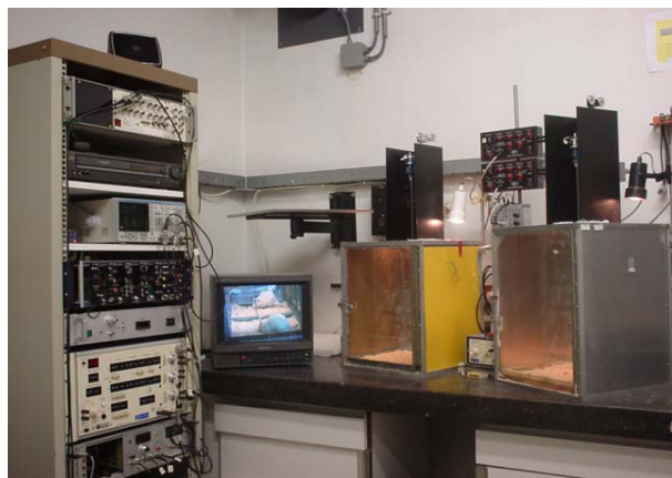
Figure 3. Experiment setup with cages with rats and the monitor receiving the image from one of the cages. On the left the stimulation generator and video recorder.
