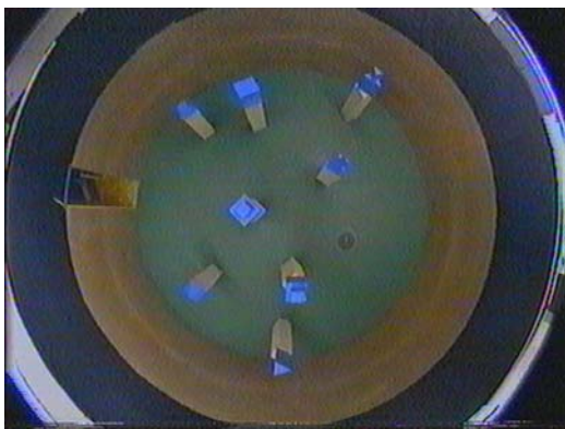
Figure 1. Camera view of the Real Arena Maze with the different geometric landmarks and the pressure sensitive platform disc on the floor.
