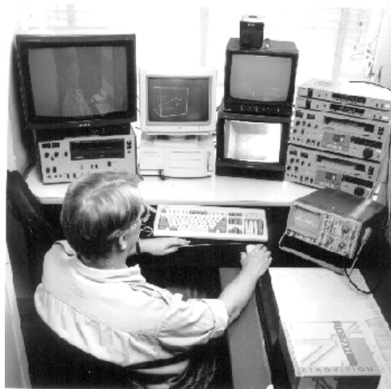
The set up for automatic recording and analysis of the flight behavior of insects in a wind tunnel. (photo courtesy of Wageningen Agricultural University)
