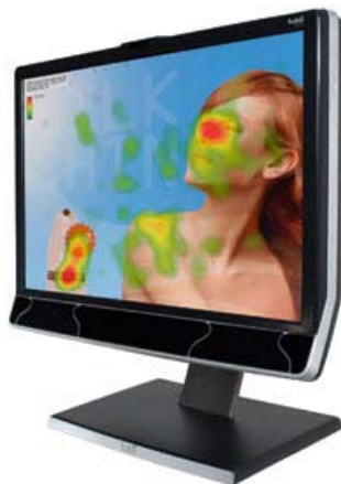
Figure 1. Hotspots on a webpage measured with a computer-monitor eye tracker.
