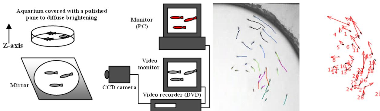
**Figure 1.** Left: Diagram of the multitracking setup. A CCD camera filmed a mirror reflecting the bottom of the circular tank. Right: example of tracks (detail of the arena, period of 1 sec) and the same image with individual assignments and velocity speed.
